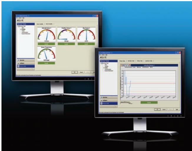
AMS Device Manager uses EDDL technology to create an asset dashboard with clear indication of device and asset status.
